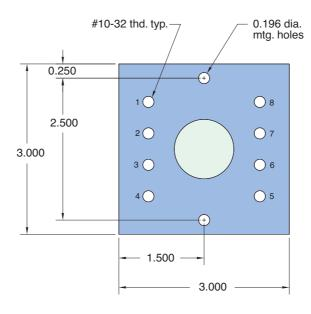
**Size:** 3" x 3" x 5/8" thick - 1 module **Use:** Provides mounting for a single
