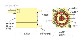
Normally-Closed 2- & 3-Way Electronic Poppet Valves with Wire Leads
