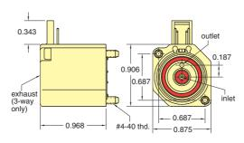
Normally-Closed 2- & 3-Way Electronic Poppet Valves with Top Pin Connector
