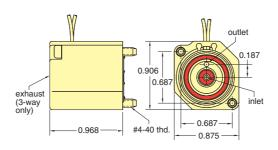
Normally-Closed 2- & 3-Way Electronic Poppet Valves with Board Mount
