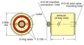
Additional Note Use only Normally-Closed 3-way pilot valves in conjunction with EVB-2/EVB-3
