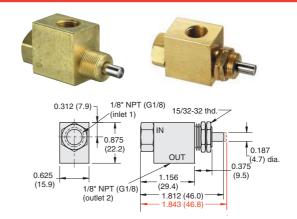
Input Pressure: MJV-2/MJV-2-MG - 300 psig/21 bar max. MJVO-2/MJVO-2-MG - 150 psig/10 bar max.
