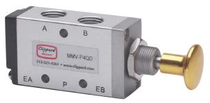
Push/Pull spool valves are available in both 3- and 4-way configurations. The Detent version maintains spool position by friction, while the Momentary spring returns to the home position.
