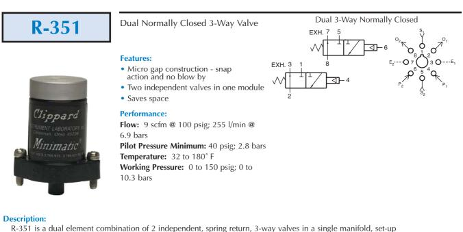
for normally-CLOSED usage only. Ports 3 and 7 are exhausts to atmosphere and cannot be restricted.
