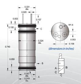
These new direct actuating valves offer an extremely fast response time for accurate dosing of minute volumes with the same long life you expect from the original Clippard EV line of electronic valves, now in a 8 mm cartridge package.
