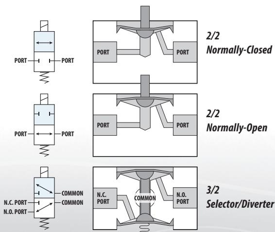
The **Clippard NIV Series Media Isolation Valve** is a solenoid-operated device that uses a flexible diaphragm to isolate the actuation mechanism from the fluid path. Media isolation valves are commonly used for a wide variety of applications, including those that require precise, repeatable dispensing of media for analytical instrumentation. All wetted areas of the valve are PTFE, making this series ideal for use with corrosive media.
